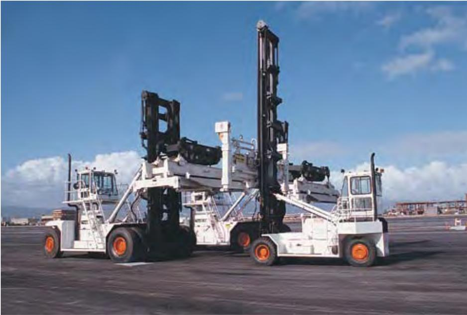
Container lift trucks readied for use at the port. Axle loads will be as high as 200,000 lbs (90,700 kg).
