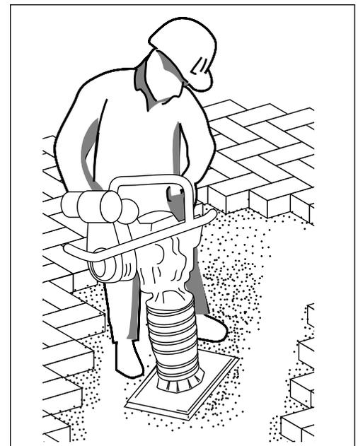
Figure 10. Compaction of the base in 2 to 4 in. (50 to 100 mm) lifts and monitoring density with a dynamic cone penetrometer or a nuclear density gauge are essential to minimizing settlement.
