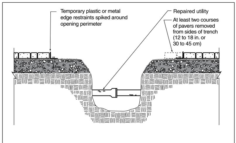
Figure 8. T-shaped cross section of the excavated opening
