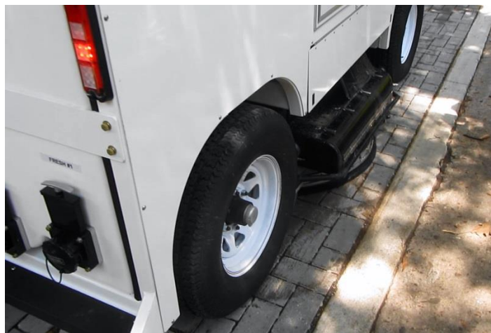
Figure 6. The Cyclone machine cleaning a PICP alley.
