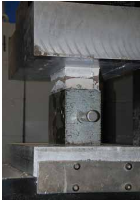
Figure 6. Left: a capped concrete paver under load in a compression testing machine; Right: a paver tested in compression; the moment it breaks is the recorded load.
