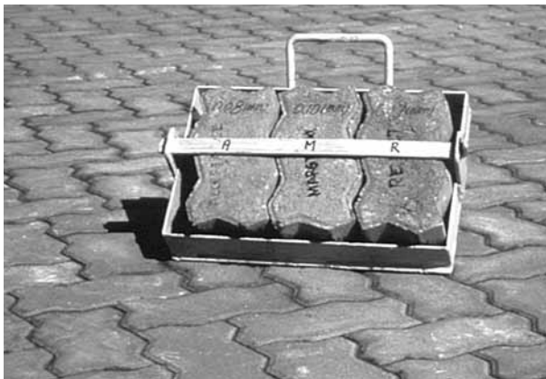
Figure 16. A simple gauge for checking dimensional tolerances on the job site.
