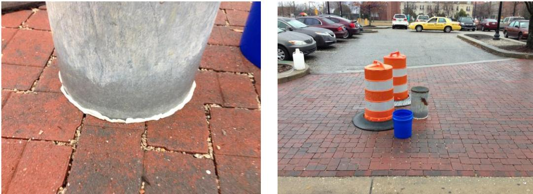
*Figure 1. Infiltration ring fixed to permeable pavement with plumber's putty (left). Testing location 3 in center of driving lane (right).*
