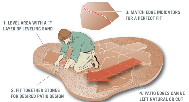
**5** After all stones are in place, cut or score and break stones to fit the desired shape. EssexStone can also be left uncut giving the appearance of a rough cut stone.
