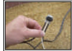
9. Once you have all three wires in each of the three holes and pushed all the way to the back, squeeze the connector with a pair of pliers to push the black cap down. This will make the connection between all three wires and will require some force. The connectors also contain silicone to protect the connection from moisture which may squeeze out on this step; be careful not to get it on your clothing.
